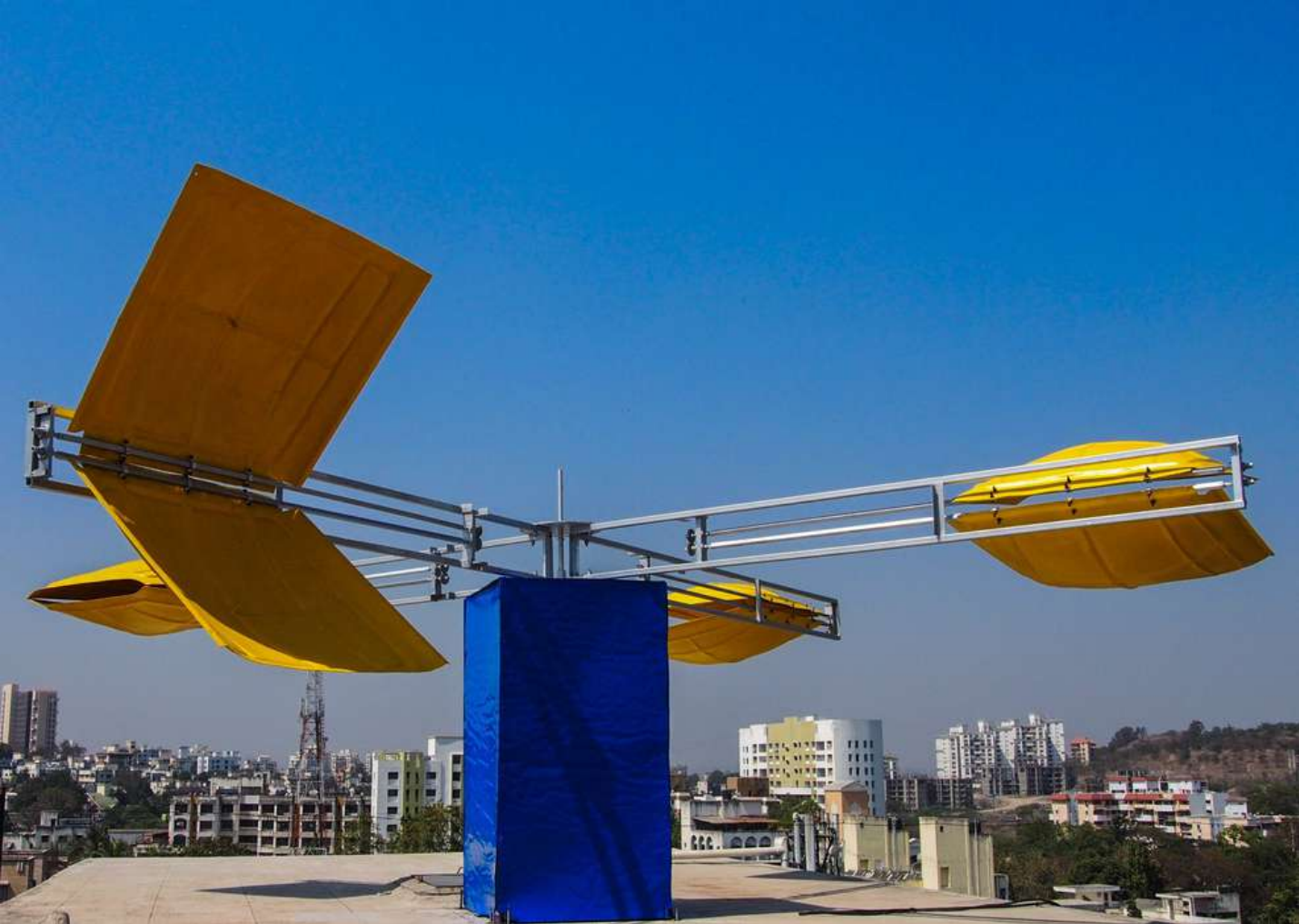
Low speed Breeze Power Mill made from recyclable waste materials (patented) Size - 14ft diameter Year - 2015
